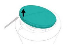
Using the opening tool, remove the upper cap.
