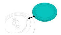
When placing the upper cap on ICO, alig the notches with the pins
