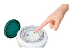
Press the button for a minimum of 5 seconds until you see the yellow LED flickering.
